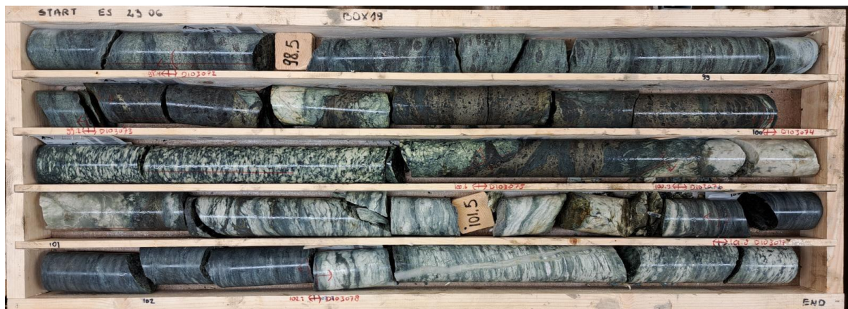
Figure 2: Hole 12 Stormyra norite banding with 0.1 to 1.0% mixed sulphides, pyrrhotite, pyrite, pentlandite and chalcopyrite.
